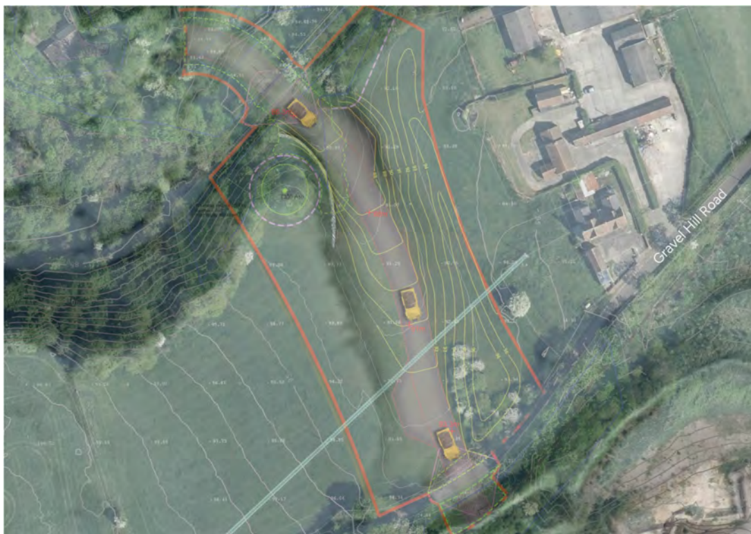
Plate 16: Proposed Development, overlain on LiDAR imagery (yellow contours relate to proposed changes)
