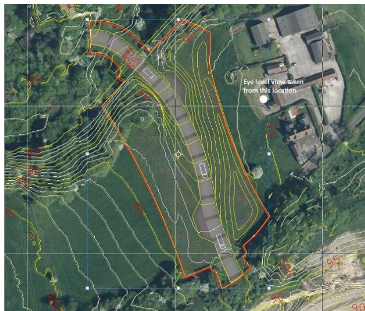
Figure 3-2: Plan showing profile of modified landform (extract from Drawing CHR-001)
