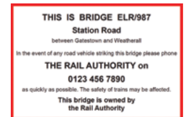
Example identification plate at rail bridge
